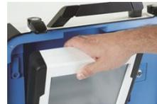
8. Seat the tablet in the cradle, tilt it back and lock it in place.
