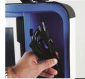
6. Plug the Verity Touch Writer (VAT) power cord into the power brick and then plug the power brick into the back of the Verity Touch Writer (flat side up). **DO NOT PLUG THE POWER BRICK INTO THE WALL YET.**
